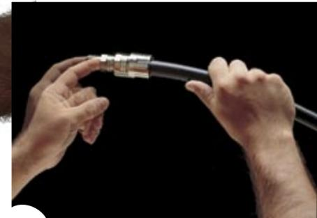
Once inserted, MegaCrimp stays inserted. It won't fall out during the crimping process.
